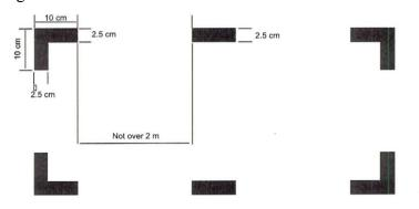
(b) If the corner markings are more than 2 m (6.5 ft) apart, intermediate lines 9 cm (3.5 in) x 3 cm (1.2 in) shall be inserted so that there is no more than 2 m (6.5 ft) between adjacent markings.
